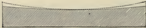
FIG. 65.—Showing in an exaggerated form how the edge of the speculum is worn down by polishing.
